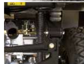
Robust, reliable semi-independent rear suspension
