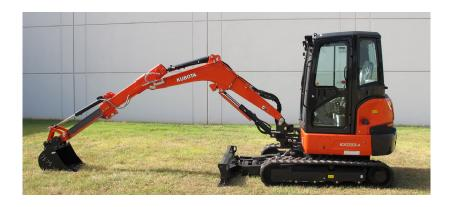
Ideal for those hard to reach areas, the KX033-4's new optional extendable dipper arm can be quickly and easily extended up to 31 inches, boosting productivity as well as efficiency.
