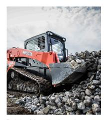
The Kubota SVL95-2s has the muscle to handle heavy-duty lifting and loading chores, and the versatility to handle a variety of other assignments.
