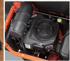
Z723/Z724/Z725 models (Powered by KOHLER° Command PRO engines) 22.5HP\*\*\*/23.5HP\*\*\*
