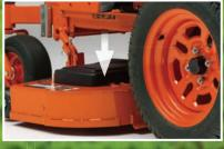
**3** Push and release the pedal again to lower the deck
