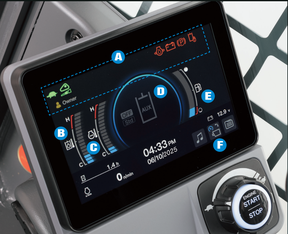
A. Situation Indicator (such as working function, battery charge indicator etc..) B. Hydraulic Oil Temperature C. Coolant Temperature D. AUX Mode E. Fuel Level F. Menu Icons
