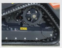
>>> Welded track frame has angled top for debris shedding and the dual flange front idler provides better stability and weight distribution.
