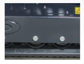
Maintenance time is reduced with permanently sealed and lubricated track rollers, and with the grease type track tension system.
