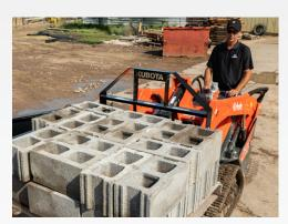
>> 1000 lbs. ROC combined with 15 gpm auxiliary hydraulic flow make for a powerful and productive compact utility loader.
