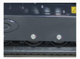
Maintenance time is reduced with permanently sealed and lubricated track rollers, and with the grease type track tension system.
