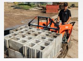
1000 lbs. ROC combined with 15 gpm auxiliary hydraulic flow make for a powerful and productive compact utility loader.
