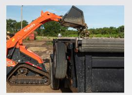
Vertical lift loader arms reach higher and further than the competition with a hinge pin height of 84.7" and a reach of 26" (at 45° dump angle).
