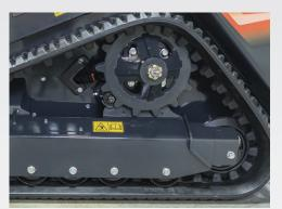
Welded track frame has angled top for debris shedding and the dual flange front idler provides better stability and weight distribution.
