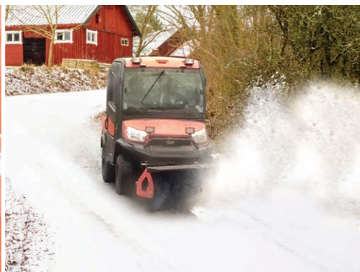
PTO powered - turns at more than 240 rpm
