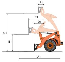
Note: The above dimensions are based on the machine with wide tires, SSL type quick coupler, standard bucket/pallet fork and ROPS/FOPS canopy and cabin.
