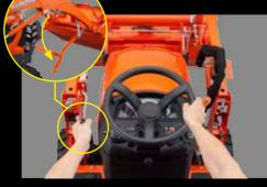
Step 1: Lift the loader boom and fully dump the bucket.
