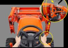
Step 4: Pull one lever to quickly and easily detach the hydraulic lines as a unit and store the coupler on the loader boom.
