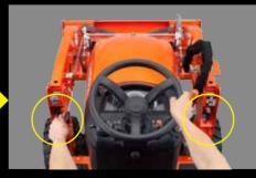
Step 2: Unlatch the loader latch levers to detach the front loader hooks.
