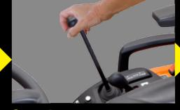
Step 3: Use the loader lever to remove the loader frame from the mast.
