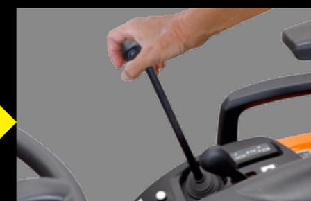
**Step 3:** Use the loader lever to remove the loader frame from the mast. Turn off the engine and move the loader joystick lever to relieve the hydraulic pressure.
