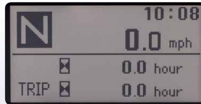
The IntelliPanel's standard indicators display the hour meter, trip meter, fuel consumption, PTO revolutions, HST information, DPF particulate matter accumulation, and maintenance information on the large and easy-to-read screen. The information can be switched easily with button operation. Furthermore, warning indicators, scheduled service alerts and DPF regeneration are also indicated on the panel to keep you informed at all times.
