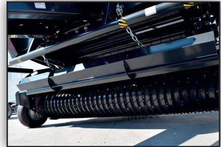
Clean raking 86" wide pick-up with twin cam tracks, 5 tine bars and roller crop press.
