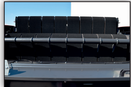
Durable MRT profile belts with heavy duty MATO lacings. Fully adjustable hydraulic density control (Optional proportional electric control).
