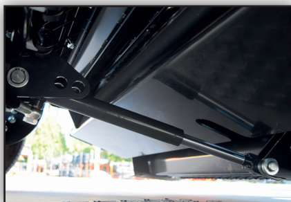
Standard fit hydraulic pick-up lift for reduced downtime between jobs and added in field convenience.
