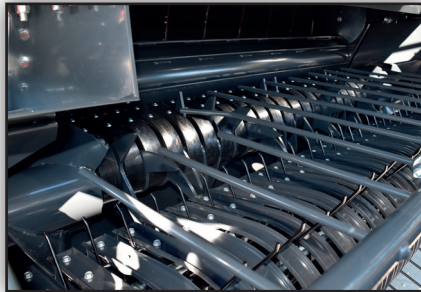
Full width rotary feeding system with huge intake capacity and gentle crop handling.
