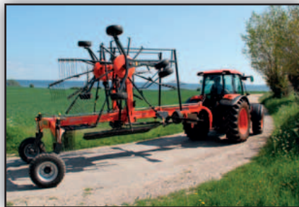
To limit transport height on RA2076 further, the tine arms can be removed. The swath board folds up automatically.
