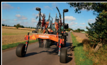
With tine arms removed, transport is as low as 11'4".
