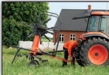
Pull type drawbar. Easy to attach.
