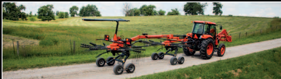
Pulled axle suspension for smooth running and reduced power requirement.
