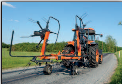
The tines are automatically leveled for added ground clearance when folding into the transport position.
