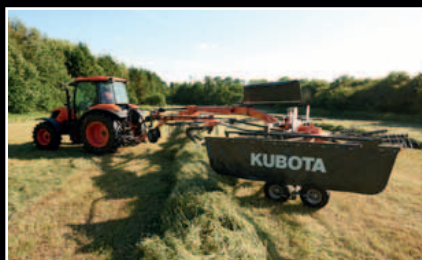
With 20" lifting height, swaths are easily crossed.
