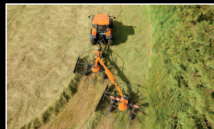
RA2071T EVO is capable of placing small night swaths for hay crops.
