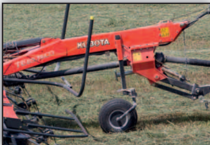
A third wheel allows for better tracking and more accurate tedding action. This wheel also helps adjust the tedding height.
