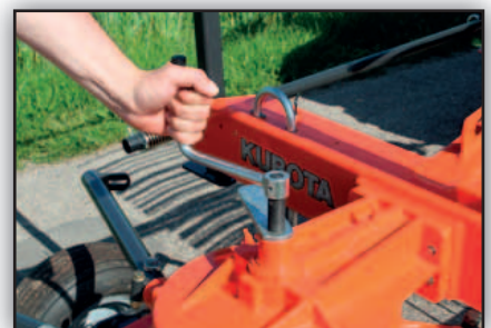
Easy setting of correct rotor height.
