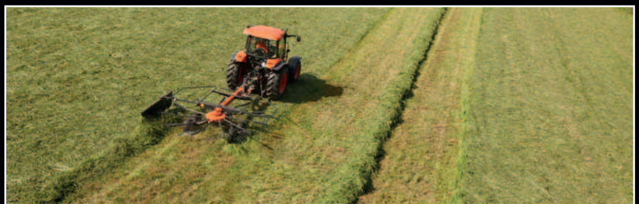
RA1042T designed for low hp tractors, while still delivering 13'9" working width.
