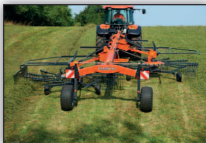
The side delivery concept allows you to collect crop from 49'3" into a single swath.
