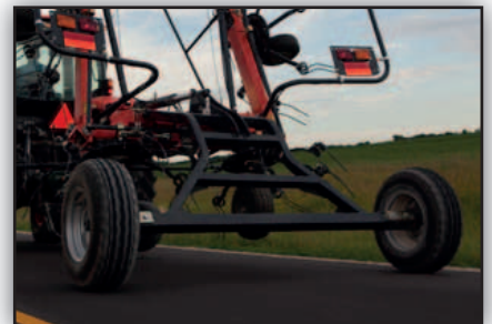
The wide track of the transport wheels ensures stability during roading of the machine.
