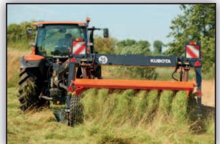
The crop is directed inwards, away from the unmowed crop.
