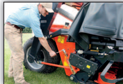
Easy adjustment of stubble height.
