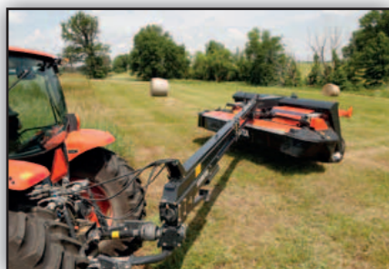
A lifting height of 18", ensures excellent ground clearance for transport and during headland turning.
