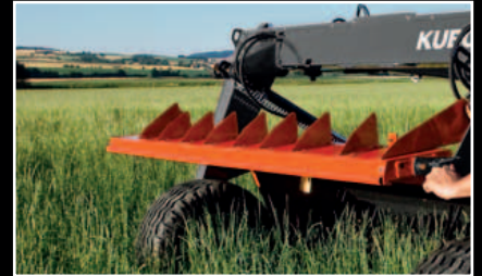
Changing from swathing to wide spreading is a one-man-job.
