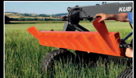
Simply turn the rear plate 180°.
