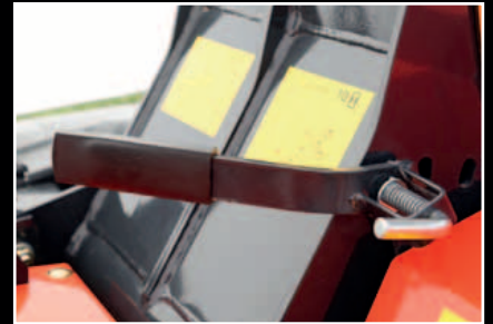
Easy adjustment of conditioning intensity.
