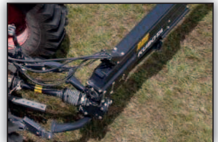
The swivel hitch headstock with reversible gearbox provides optimal maneuverability.
