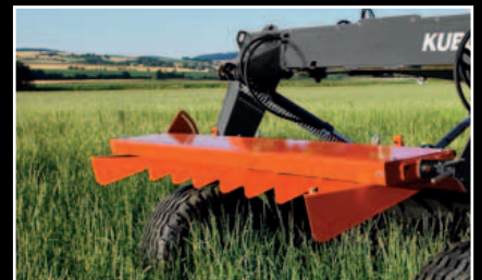
Dismount the two deflector doors and you are ready to mow.
