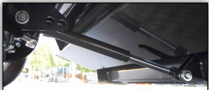
Standard fit hydraulic pick-up lift for reduced downtime between jobs and added in field convenience.
