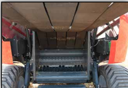
Bale formation belts are equipped with industry leading MATO lacings.
