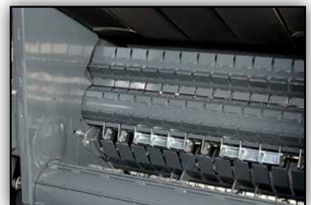
The two front rollers with self-cleaning scrapers are designed to work well in silage and provide instant bale formation.
