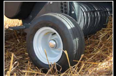
Guide wheels with large flotation tires are fitted as standard equipment.
