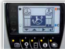
Max. Oil Flow Setting (AUX1 and AUX2)
