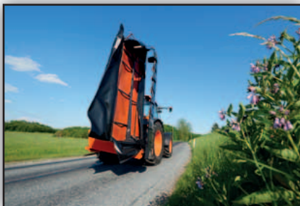
For transport, the machine can be folded hydraulically from the tractor cab to the vertical transport position, well behind the tractor, ensuring a stable and steady transport.
