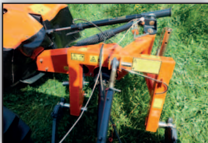
Hitch is very easy to attach, while the parking lock keeps the headstock in level position.
