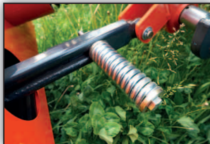
Spring loaded BreakAway.
