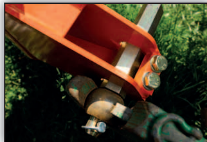
The linkage pins are easily adjusted to match the tractor width, which enables the mower to cut to its' full working width.
